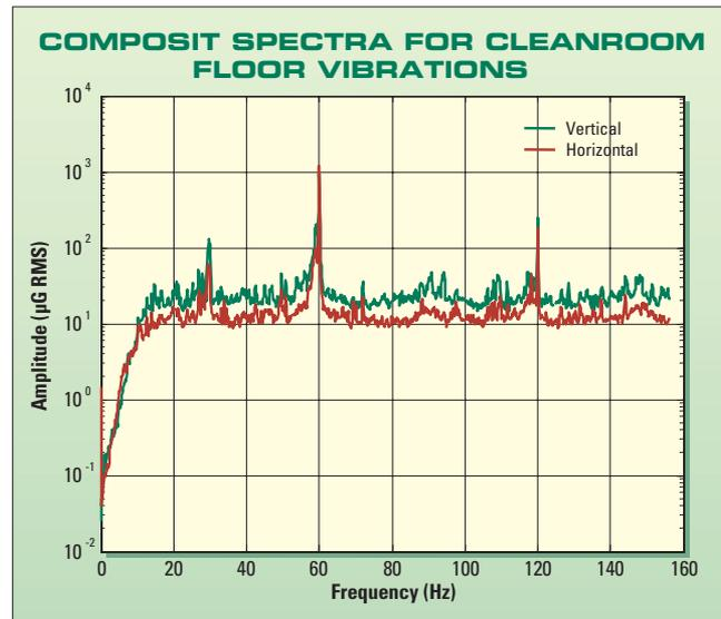
**2.** These composite spectra for cleanroom floor vibrations were compiled using measurements from more than 20 cleanroom sites. Large vibration amplitudes are seen at multiples of 30 Hz, which can be traced to frequencies generated by common cleanroom equipment.
