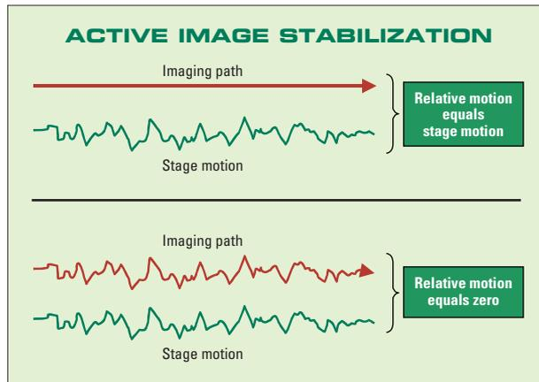
**4. Active image stabilization by beam deflection is one way to maintain a stable image path.**
